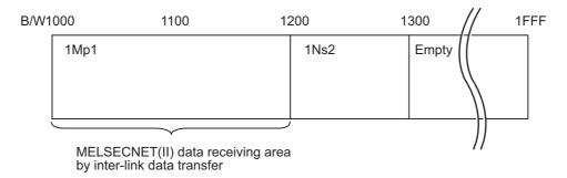
When the data is transferred from MELSECNET(II) to MELSECNET/10, B/W1000 to 11FF shall be the transfer area.
