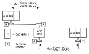
(2) Up to four repeater units can be used in a single network.\*2
