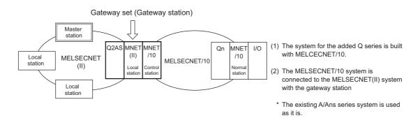
Since QCPUs are incompatible with MELSECNET(II), the network system is built in MELSECNET/10 by adding a gateway station to the existing MELSECNET(II) network system.
