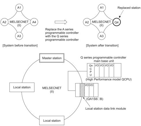
By mounting the local station data link module, the QCPU replaced by the A/AnSCPU can communicate as the local station without changing the existing network link assignment even after CPU replacement.
