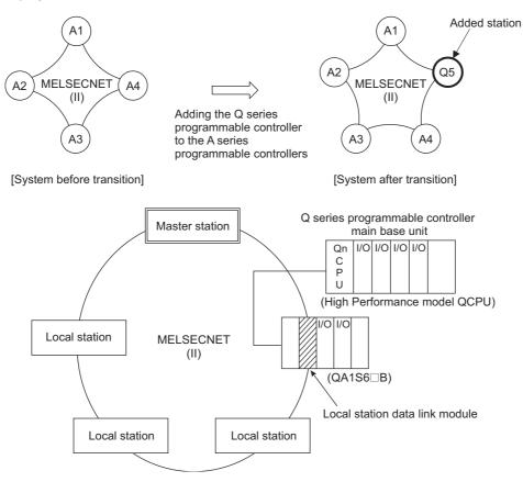
When the QCPU is added to the existing network, it can communicate as the local station using the existing network link assignment by mounting the local station data link module.
