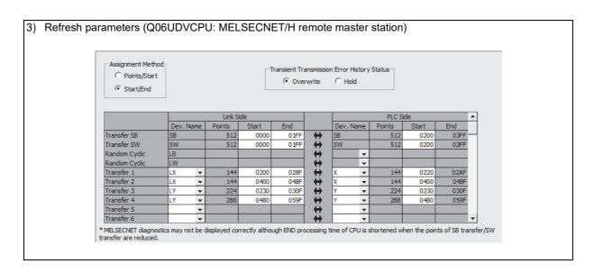
An overall picture of CPU-side device assignments on the Q06UDVCPU to which the PLC to PLC network (control station) and remote I/O network (remote master station) is mounted can be checked at [Assignment image diagram] in the GX Works2 or GX Developer network parameters. After setting the parameters, make sure that assignments are correctly set.
