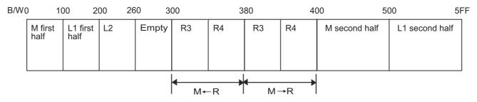
3) BW network range assignment after addition of the gateway station (L5/1Mp1) (Assignment in the area of 200 to 3FF is W only.)
