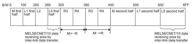
When the data is transferred from MELSECNET/10 to MELSECNET(II), B/W260 to 3FF shall be the transfer area.
