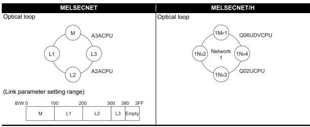
A MELSECNET/H module set as normal station requires network parameter setting. For replacement of MELSECNET (II) module mounted on the CPU module of the AnN/AnA/AnSCPU (excluding AnUS(H)CPU), newly set network parameters.
