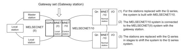
The system is shifted to the MELSECNET/H(10) network system by replacing A/AnS/QnA/QnASCPUs in the existing MELSECNET(II) network system with QCPUs in stages until all CPUs are replaced by QCPUs.
