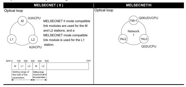
A MELSECNET/H module set as normal station requires network parameter setting. For replacement of MELSECNET (II) module mounted on the CPU module of the AnN/AnA/AnSCPU (excluding AnUS(H)CPU), newly set network parameters.
