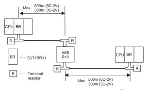
(2) Up to four repeater units can be used in a single network.\*5
