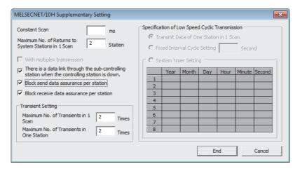
(b) BW first half/second half assignments in the MELSECNET II mode and composite mode Set the station inherent parameters of the MELSECNET/H to all stations to re-use MELSECNET II sequence programs more efficiently.
