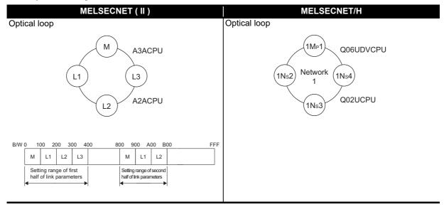
Each of the MELSECNET II first and second half settings correspond to [Setting1] and [Setting2] set to all stations according to the "Station inherent parameters" on MELSECNET/H. (Example) Station inherent parameters of a normal station (1Ns2)
