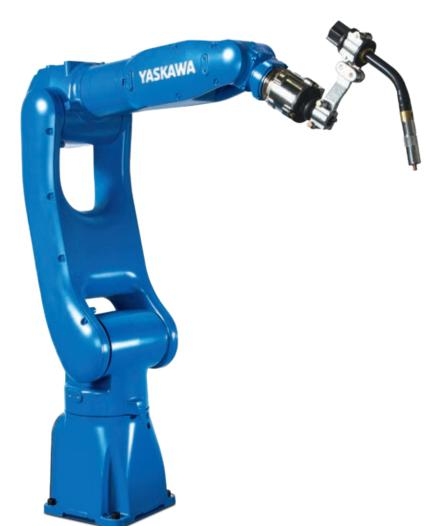
The MOTOMAN AR900 is a compact high-speed 6-axis robot which provides accurate performance to achieve optimal results in extremely difficult conditions and especially for the high demands of arc welding applications.
