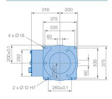
Mounting options: Floor, ceiling, wall, tilt\* Protection class: Main axes (S, L, U) IP54 (option IP65), wrist IP67
